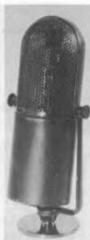
FIG. 14. RCA-77A unidirectional microphone with cardioid pattern designed by H. F. Olson and first used in 1933.
