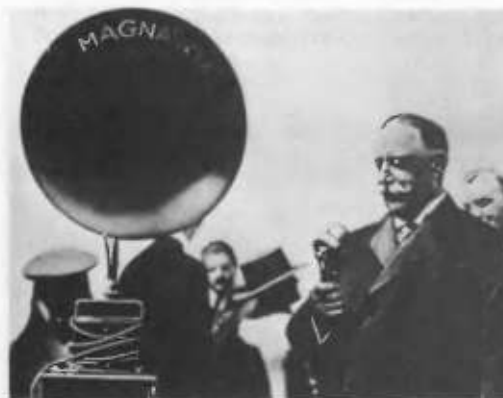
FIG. 1. Edison Amberola phonograph horn connected to Pridham moving coil telephone receiver used to transmit speech that could be heard two blocks away.
