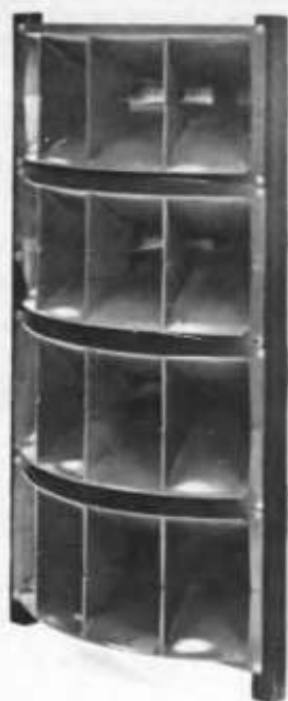
FIG. 15. Directional array of sectorial horns to provide limited vertical beamwidth and wide horizontal beamwidth in the frequency range above 500 Hz.
