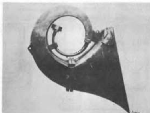
FIG. 10. 555-W receiver attached to 70-Hz cutoff coiled horn used in first sound motion picture theaters.
